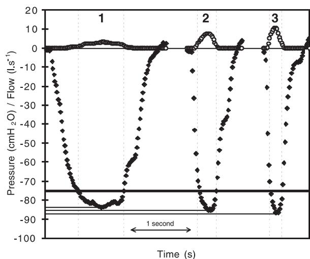
**Figure 4** A series of plots illustrating the effect of flow rate upon pressure profile, using the threshold device on a  $-75$  cm H<sub>2</sub>O setting. ◆, pressure; ○, flow.
