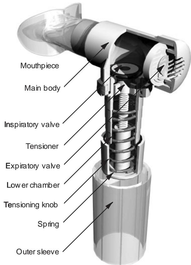
Figure 2 Cut-away illustration of the finalised pressure threshold training device.
