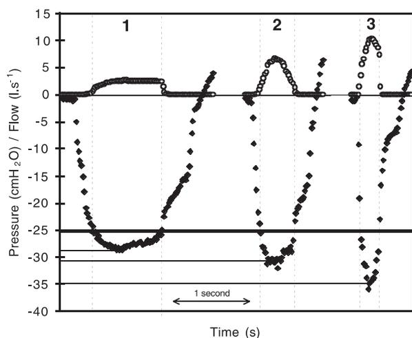
**Figure 3** A series of plots illustrating the effect of flow rate upon pressure profile, using the threshold device on a  $-25$  cm H<sub>2</sub>O setting. ◆, pressure; ○, flow.
