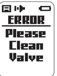
If the valve head becomes clogged with dirt or saliva then the POWERbreathe unit cannot function correctly and an error message may be displayed. When this happens, you should follow the cleaning instructions detailed in section 10.1
